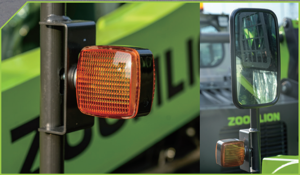
Optional turn signals and exterior rearview mirrors They do not move with the lift arm, making it easy to observe the situation at the back of the machine at any time and keeping you safe.
